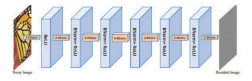
Fig. 4. The architecture of IRCNN
